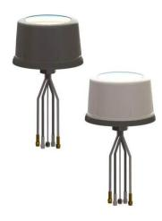
The Laird Connectivity vehicular five-port MIMO antenna covers the 698-960/1710-2700 MHz and 2300-2700/4900-5900 MHz frequency ranges with an added global navigational antenna. Configured with two 3G/4G ports and two dual band Wi-Fi ports and a fifth port configured with a GNSS navigational antenna.
