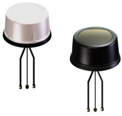
The Laird vehicular 3-port MIMO antenna covers the 698-960/1710-2700 MHz, as well as GPS (1575.42 MHz) frequency ranges. Configured with 2-port, dual-band elements in addition to 1-port with integrated GPS.
