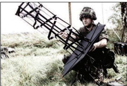
Full Band Single-Unit Antenna across the 240-400 MHz frequency
